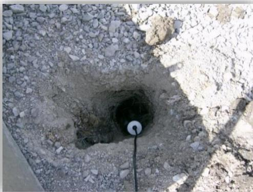
*Packages include coupons which are linked to the communication system allowing for instant pipe to soil potential readings.*
