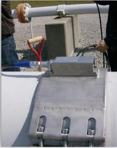
Guided Long Range Remote Monitoring has the ability to access difficult areas in order to identify internal and external corrosion threats in pipelines.
