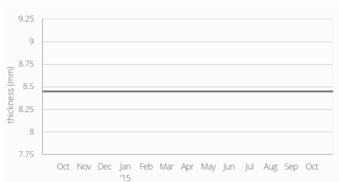
**Figure 9** Typical spotOn® U thickness output
